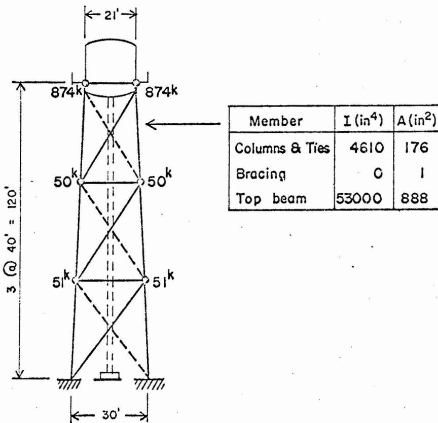
Fig.7 Elevated water tank, Structure No.5.
