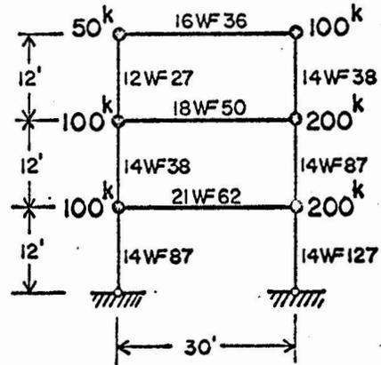
Fig.3 Three storey frame, Structure No.1.
