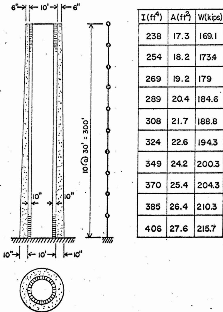
Fig.9 Reinforced concrete smokestack, Structure No.7.
