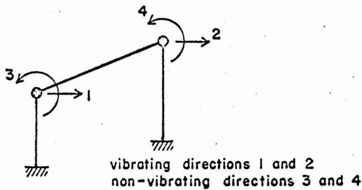
Fig.1 Deformation numbering.
